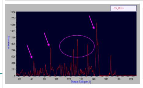
The spectra illustrated here were obtained with the Dimension-P1<sup>TM</sup> using the LSI External Sampling Module. The sampling module was heated from 25 to 85° C. The spectra were averaged 5 times and background-removed using LSI RamanSoft<sup>TM</sup>. The spectra shown are actual RamanSoft<sup>TM</sup> screen shots. The Dimension-P1<sup>TM</sup> was configured for a coverage of 140 -2070 cm<sup>-1</sup> at 3 cm<sup>-1</sup> resolution.
